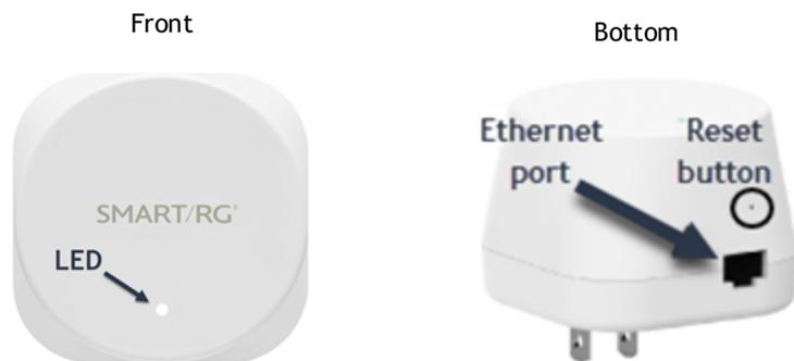
The **Reset** button is used to reset the device to factory default settings. Resetting the extender also unpairs it from the hub gateway. Press the button until the LED blinks green (about 15 seconds) to initiate reset.
